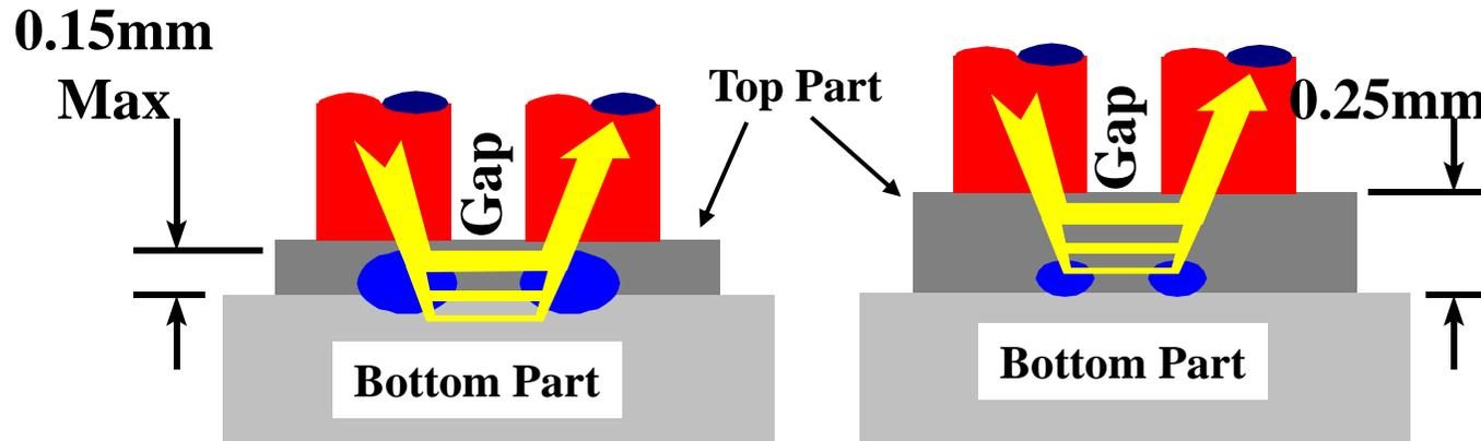
Limited to 0.15mm(.006in) thickness
